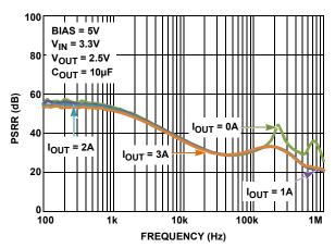
FIGURE 28. BIAS PSRR vs LOAD CURRENT
