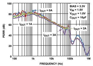
FIGURE 29. V<sub>VIN</sub> PSRR vs LOAD CURRENT
