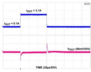
FIGURE 26. 3A LOAD TRANSIENT RESPONSE
