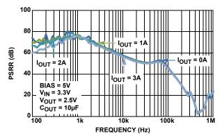
FIGURE 3. V<sub>IN</sub> PSRR vs LOAD CURRENT (ISL80113)
