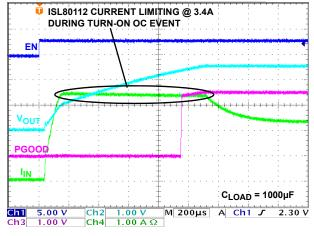
FIGURE 21. ISL80112 ENABLED INTO OVERCURRENT
