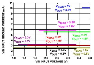
FIGURE 13. INPUT GROUND CURRENT vs  $V_{IN}$  and  $V_{OUT}$
