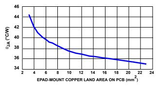
FIGURE 37. 3mmx3mm-10 PIN DFN ON 4-LAYER PCB WITH THERMAL VIAS  $\theta_{JA}$  vs EPAD-MOUNT COPPER LAND AREA ON PCB
