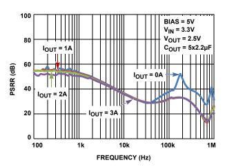
FIGURE 34.  $V_{\mbox{\footnotesize BIAS}}$  PSRR vs LOAD CURRENT
