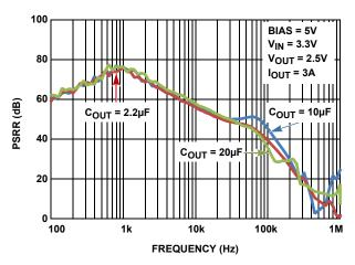
FIGURE 31. VIN PSRR vs COUT
