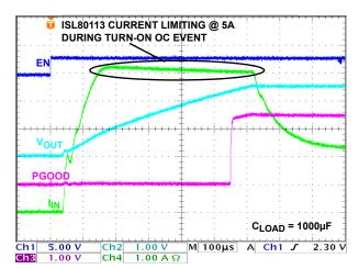
FIGURE 22. ISL80113 ENABLED INTO OVERCURRENT
