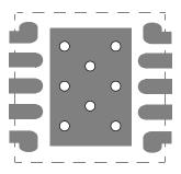
FIGURE 38. PCB VIA PATTERN
