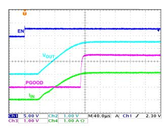
FIGURE 18. ENABLE START-UP WITH PGOOD
