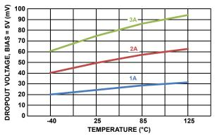
FIGURE 2. DROPOUT VOLTAGE OVER-TEMP AND IOUT
