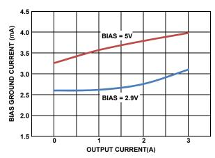
FIGURE 12. BIAS GROUND CURRENT vs LOAD CURRENT
