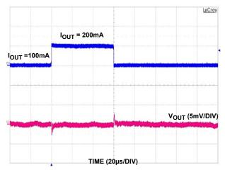
FIGURE 23. 100mA LOAD TRANSIENT RESPONSE
