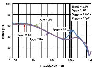
FIGURE 30. VBIAS PSRR vs LOAD CURRENT
