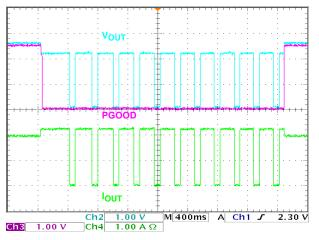
FIGURE 19. ISL8011X INTO AND OUT OF THERMAL SHUTDOWN
