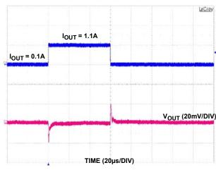
FIGURE 24. 1A LOAD TRANSIENT RESPONSE
