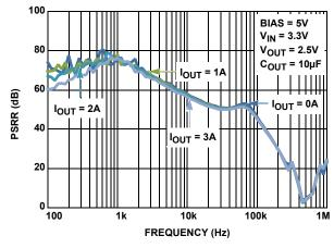
FIGURE 27. VIN PSRR vs LOAD CURRENT
