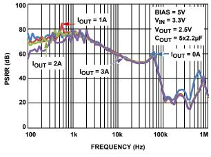
FIGURE 33.  $V_{\text{IN}}$  PSRR vs LOAD CURRENT
