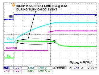
FIGURE 20. ISL80111 ENABLED INTO OVERCURRENT
