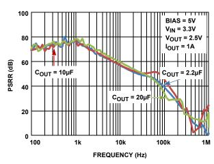
FIGURE 32. VIN PSRR vs COUT
