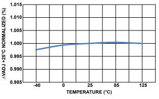
FIGURE 4.  $\Delta V_{ADJ}$  vs TEMPERATURE
