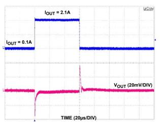
FIGURE 25. 2A LOAD TRANSIENT RESPONSE
